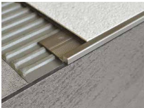
Technical and design profiles for edge protection and termination of steps of thin tile. They protect the edge of the steps from mechanical impact that could compromise the tightness of the materials that make up the tread and riser of the step. The FVT stair nosing is designed to be applied prior to the installation of the tile; the clean shape makes it minimalist and modern.
